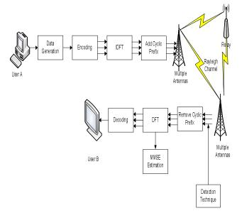
Fig. 1. Block Diagram of MIMO Detection technique.
