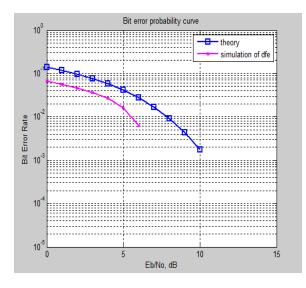
Fig. 3. BER plot of 2x2 MIMO Adaptive DFE.
